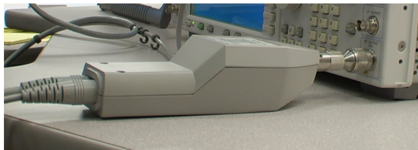
Figure 2-3 Connecting the Sensor Module to the UUT
